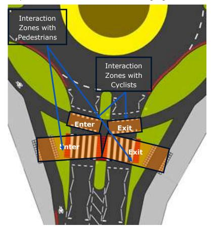
Figure 5: Interaction zones used in M27
