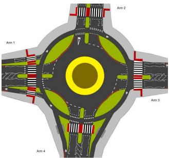
The segregated cycle track is used to keep cyclists away from circulating vehicular traffic. While this forms part of the system of segregated cycle tracks commonly used in the Netherlands, it is also used at roundabouts in urban environments where cyclists typically share roads with other traffic.
