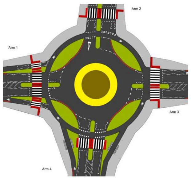
Figure 4: Layout of the Dutch style roundabout with UK markings
