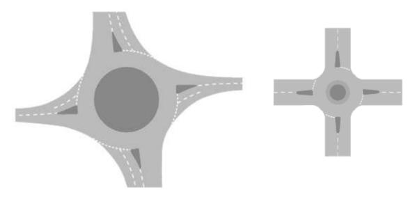
Figure 1: Comparison of UK Standard (left) and Continental (right) roundabout geometries
