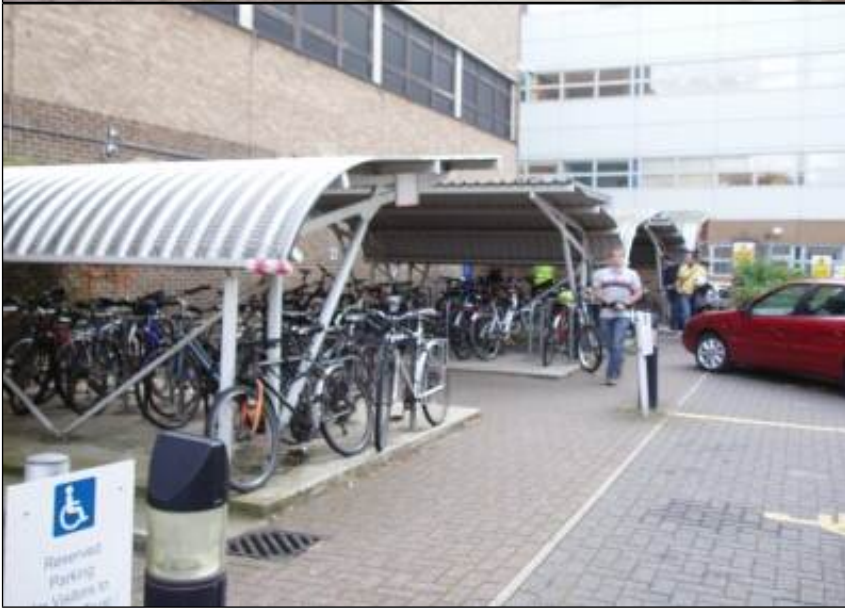
i) Front of Outpatients. Toast racks with inadequate 70cm spacing.
